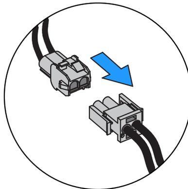
When the new igniter is in place, pull the wires inside the stove to bring the connector back into place.
