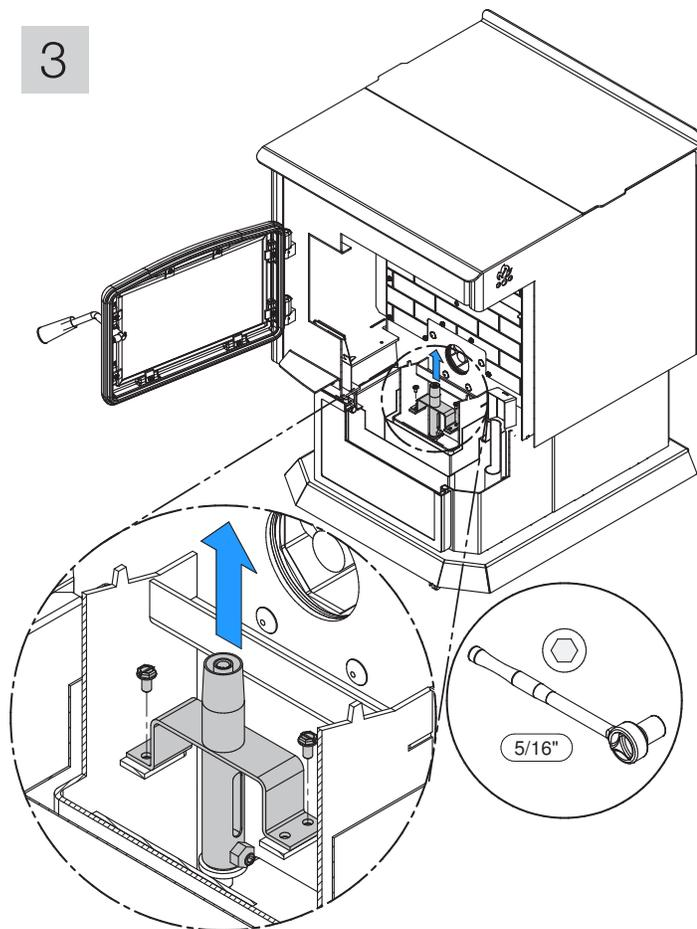
Pull the igniter upwards to gain access to the connector
