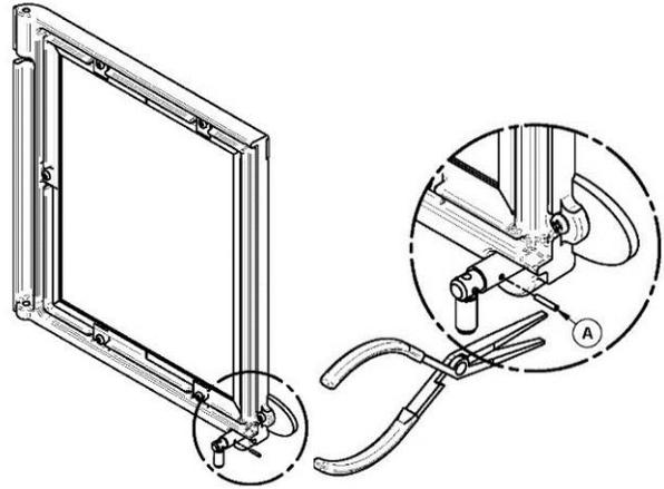
2. Turn the handle counter clockwise one turn to increase pressure. To reduce the pressure, when installing a new gasket for example, turn clockwise.
