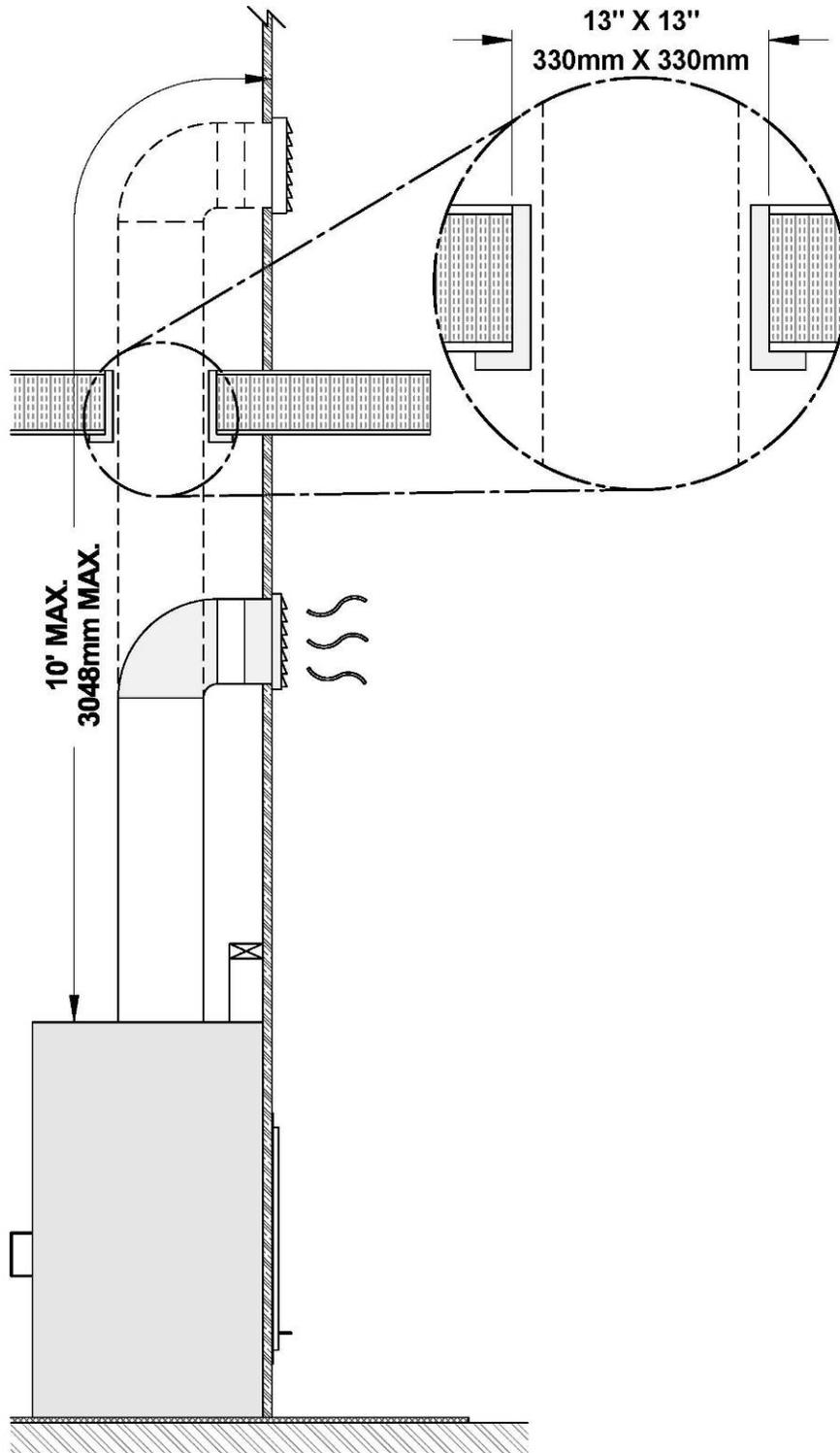
1. It is recommended to wear gloves to perform this procedure. Remove the plates closing up the 8" dia. holes on top of the fireplace. Then, cut and remove the insulation in order to obtain two 8" dia. openings. Then, remove the plates closing up the 8" dia. holes inside the fireplace.
