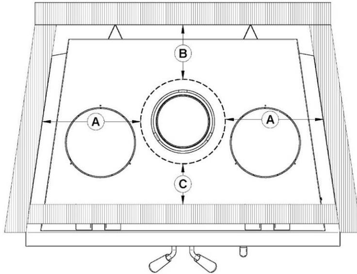
For example, for the next installation, the chimney cannot be closer to the combustible materials than the value **(A)**. Therefore, the enclosure should be X inches wider than what is suggested in the installation section, to maintain the required clearance.
