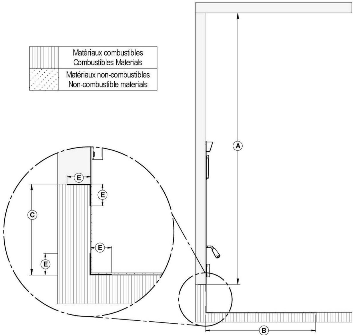
**6.3.4.2 On the floor or on a raised base less than 4"**
