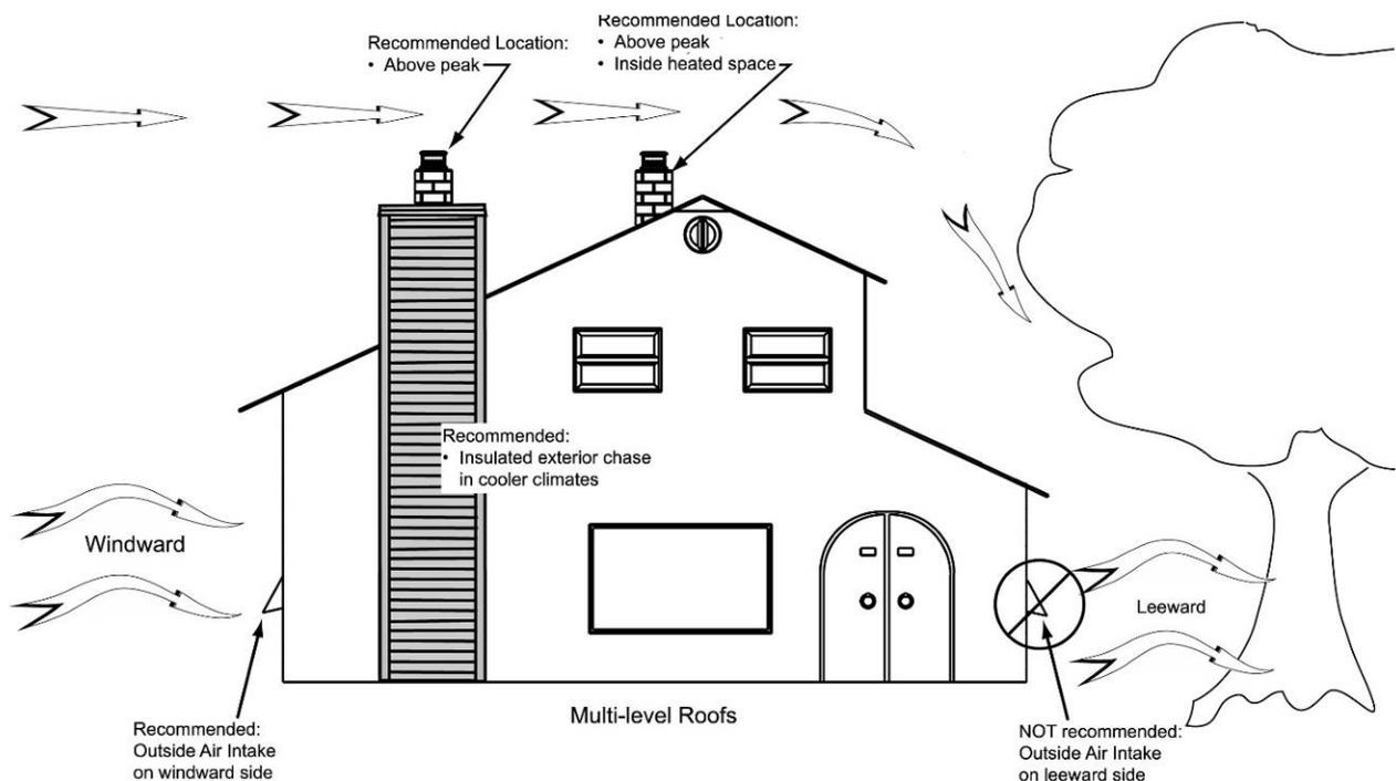
In some windy conditions, negative pressure at the duct weather hood outside the house wall may draw hot exhaust gases from the fireplace backwards through the duct to outdoors.
