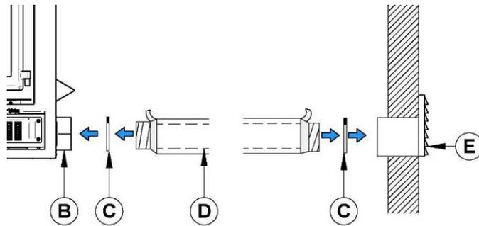
\*For a pipe length less than 20 ft., use a 4" pipe diameter. For a pipe length of more than 20 ft., or having more than two deviations, use a 5" pipe diameter. The maximum pipe length is 30 ft. (9 m).
