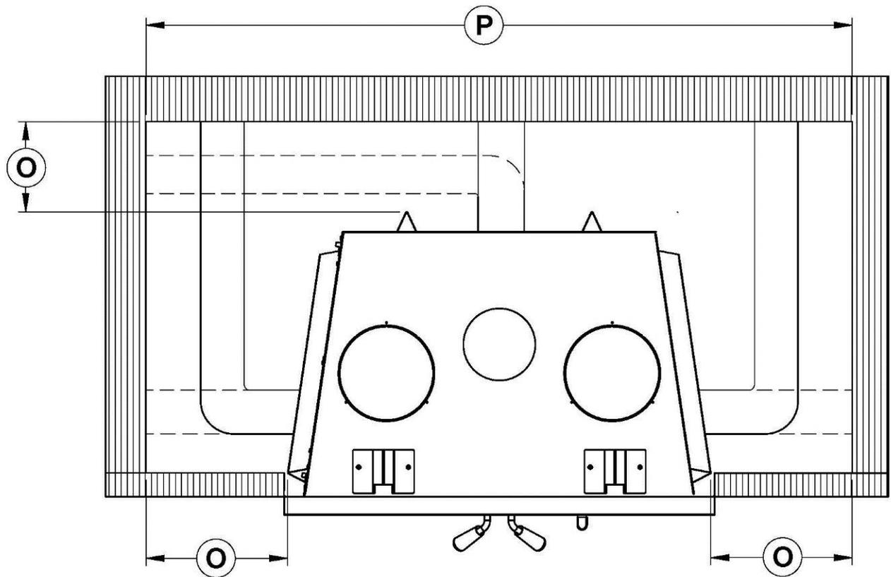
The framing dimensions are for reference only. These are recommended measurements to avoid duct to be within the standoff and have too sharp pipe angles. Smaller dimensions may be obtained depending on pipe size, type or run configuration.
