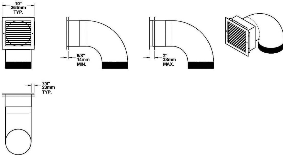
The hot air grilles can be installed in the same room as the fireplace, or one or both of the grilles can be installed in adjacent or upper rooms. Installing the ducts at different elevations will tend to exhaust more heat out of the higher grilles.
