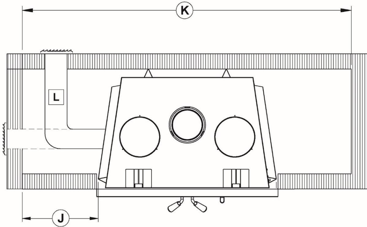
The framing dimensions are for reference only. These are recommended measurements to avoid fresh air duct to be within the standoff and have too sharp pipe angles. Smaller dimensions may be obtained depending on pipe size, type or run configuration.
