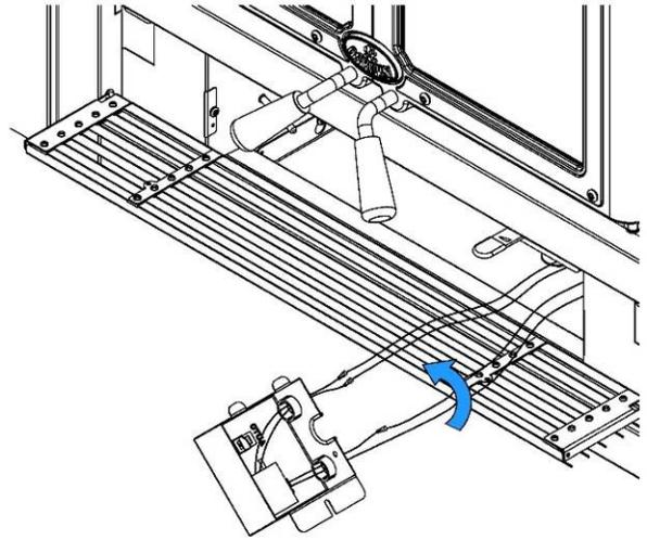
Unplug the wires. Also unplug the wire located on the terminal by removing the screw holding it in place.
