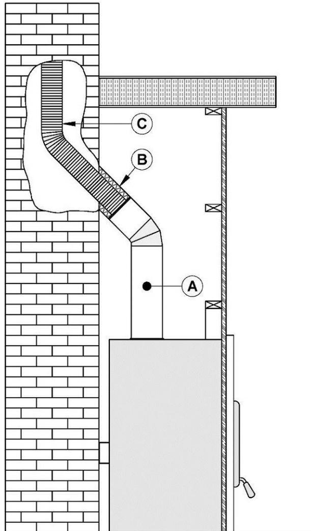
**Note:** Make sure the liner exceeds at least 12" (30 cm) the top of the masonry chimney.
