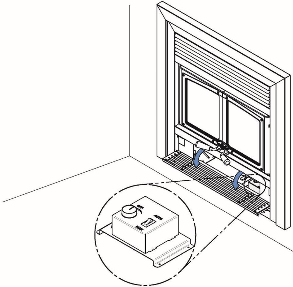
The EVEREST fireplace is equipped with a blower and a control box, accessible by pulling down the lower louvre of the faceplate.
