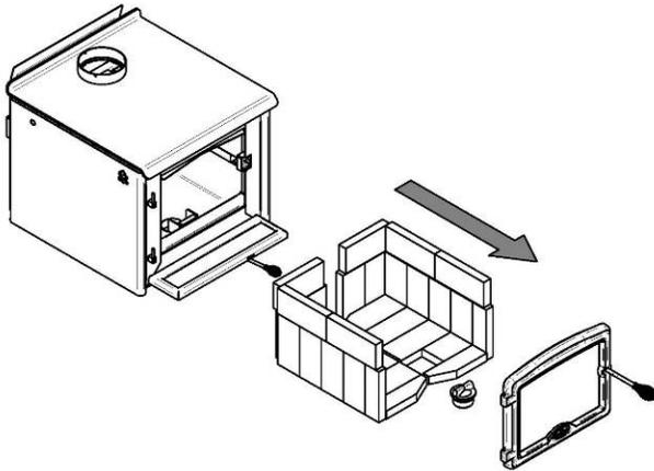
1- Remove the firebricks, the ash dump plug and the loading door from the stove to avoid breaking any parts and facilitate handling in the following steps.
