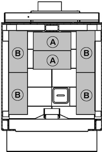
For transportation purpose, the top bricks have been laid on the bottom of the firebox. It is mandatory to install them on the brick supports before you operate the stove. **Failure to install the bricks as describe bellow may result in stove damage and will void warrantee.**
