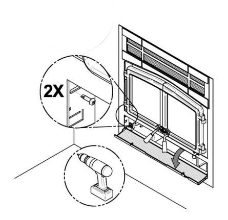
3. Attach the springs at the bottom of the faceplate into the rings of the lower louver provided for this purpose.
