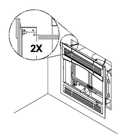
2. Firmly push the faceplate to the fireplace in order to secure the bottom with 2 self-tapping screws provided with the fireplace owner's manual.
